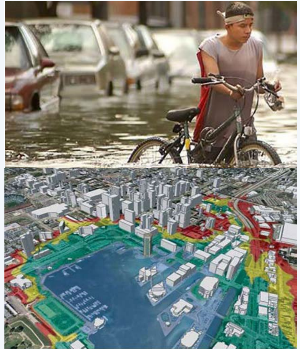
Storm surge potential with Sea Level Rise for Category 1 (blue), Category 2 (green), Category 3 (yellow), and Category 4 (red) hurricanes in the Baltimore Inner Harbor. Source: USACE Storm Surge Modeling
